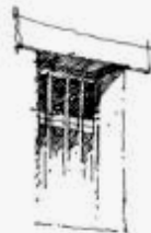
RECESSED WINDOWS PROVIDE SHADE AND EVOKE TRADITIONAL ARCHITECTURE
